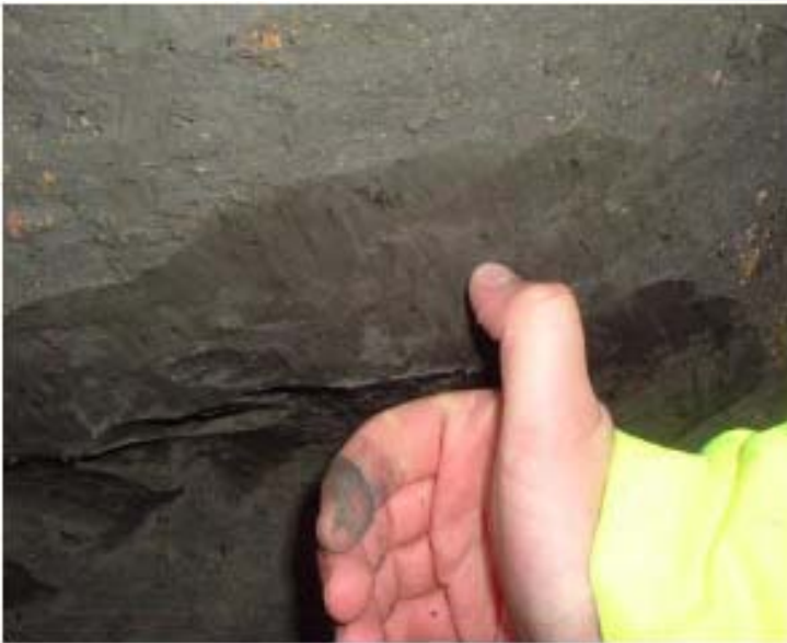
Soil Mixed Column at 5 Days
